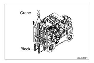
While supporting lift chains, remove the split pin and nuts from the anchor bolt. Slide out chain anchor bolt from the chain anchors of stationary upright.
